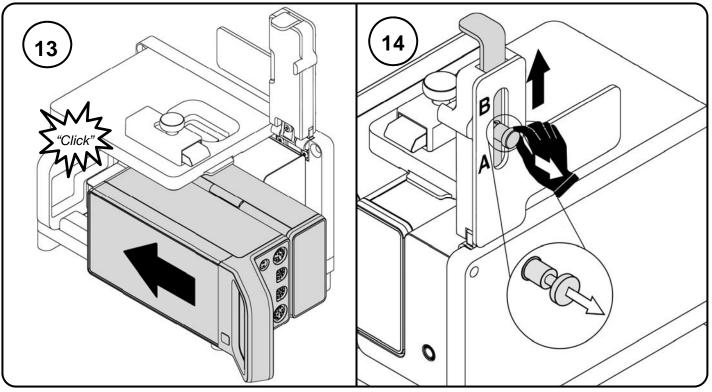
To install the IntelliVue X3 with the extension to the dock on the ambulance mount, slide the monitor from right to left until a *click* is heard that ensures a proper secure fit.
