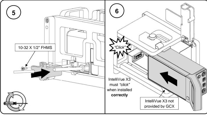
Install the provided cable retainer on the bottom of the ambulance mount using the provided 10-32 X 1/2" FHMS and a Phillips screwdriver. Make sure the screw is proper inserted to prevent cable failure. While the lever is in open position, slide in the IntelliVue Monitor from the right to left. A "click" noise ensures a safe lock to the Docking station. Make sure the Monitor is docked correctly, otherwise the mount will not properly close and may lead to device failure.
