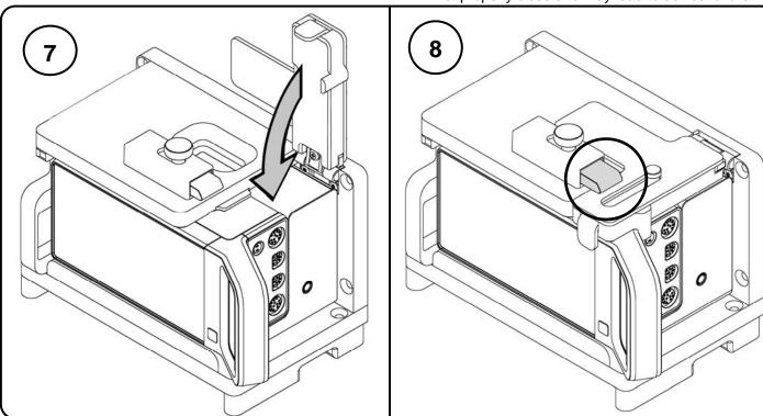
To secure the device, close the latch until end position is reached and the locking feature has secured the latch. No need to open the release button, while closing the latch.
