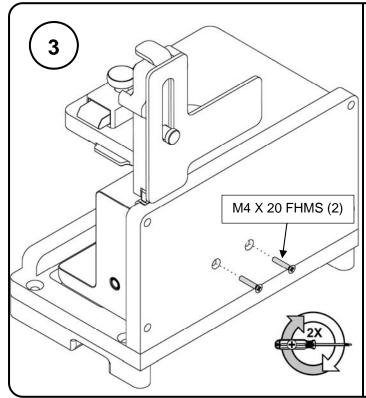
Using a Phillips screwdriver, screw in the provided M4 X 20 FHMS to the back of the ambulance mount. Make sure to correctly align the holes to ensure exact fit.
