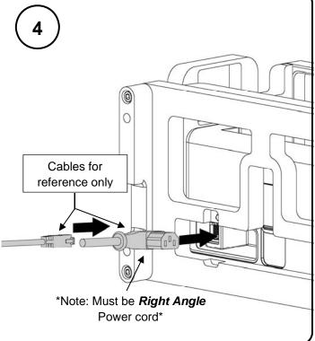
Securely install a **right angle** power cable and Ethernet cable into their corresponding slots. Failure to securely install the cables will result in connection issues and in-proper fit.
