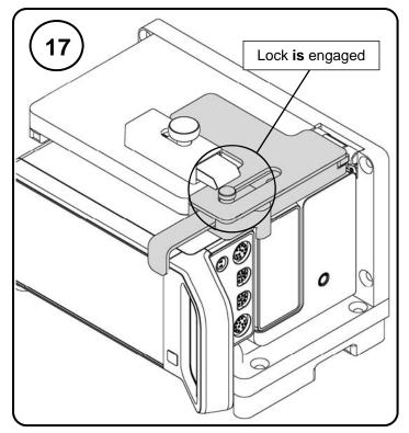
The image shown above is an example of a latch that **is** securely engaged and properly secures the monitor from moving around.
