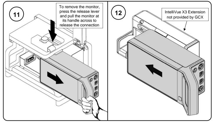
To release the Philips IntelliVue X3, Monitor from the Dock, press the release button on the top of the ambulance mount while simultaneously pulling the monitor from left to right until fully clear of dock.
