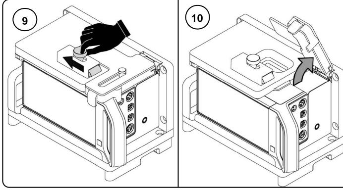
To remove the Philips IntelliVue, disengage the release button by sliding the button from left hand side until end position. Keep this position.
