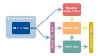
A ST 21110 device will typically expose status conditions to a broadcast control system and monitoring system, sometime via different methods.
