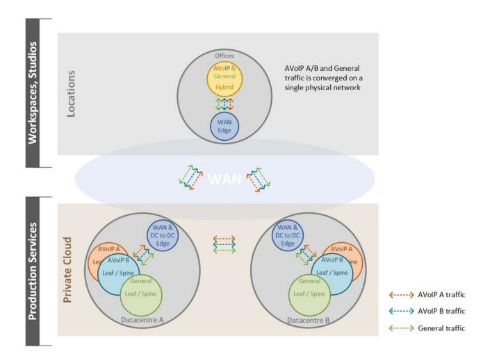
Within a region, control and AVoIP traffic is converged on a single network. The network is virtualised and dedicated AVoIP uplinks between switches create A and B networks and carry ST 2110 traffic. Resilient, GPS locked PTP GMs provide ST 2059 profile PTP to network fabrics. Each leaf will be configured as a Boundary Clock (BC). BC's shall select the best clock to lock to. Endpoints shall lock to the local BC.
