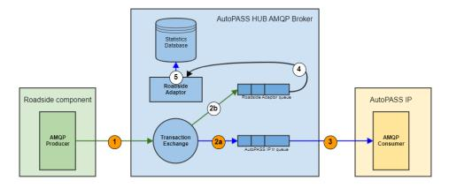
The figure illustrates how the Roadside Component (to the left) and AutoPASS IP (to the right) integrate with the AutoPASS HUB (in the middle) and shows a typical, successful scenario where the Roadside Component sends transaction data to AutoPASS IP.
