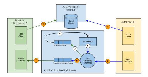
The figure illustrates how the Roadside Component and AutoPASS IP integrate with the AutoPASS HUB and shows a typical, successful scenario where Roadside Component A receives a status file from AutoPASS IP.
