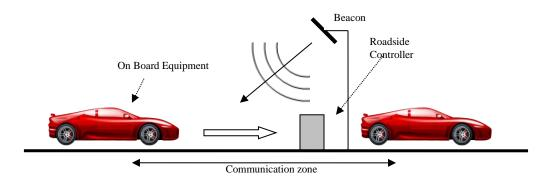
The beacon in the EFC lane continuously emits a DSRC microwave signal (5.8 GHz). When an OBE enters the communication zone of the beacon it is awakened (normally it sleeps to increase the battery lifetime) and responds by transmitting its credentials (who am I, who has issued me etc.).
