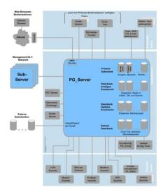
The ProGrafNT Monitoring System (SCADA) is a databased System running on Windows. All requirement for usage under GMP Conditions are implemented and qualified. Audit trail, User Management, data storage, visualisation and trending are state of the art.
