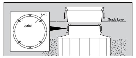
Adjust knobs to set the frame to stringline level, adjust for fall in grade. Set the frame 10mm above grade level.
