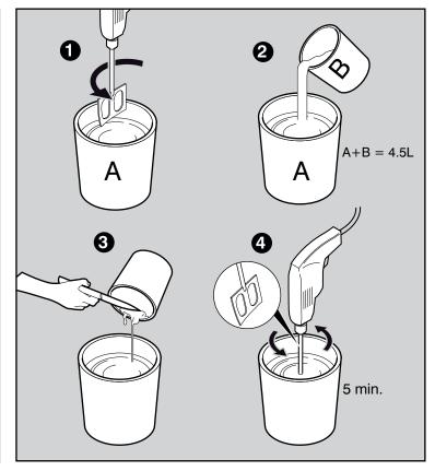
1 set of cans A+B will seal 2 sumps. Decant mixture from can A into can B to have more control when puring the mixture into the void, onto the sand base. Avoid spilling the contents to ensure a clean finish on the side walls of corbel and skirt. The sealant shall be poured to level 30mm below the top edge of the Corbel (the amount of sealant required is dependant on the height of the system but should be between 1.5 and 1.7 Litres).
