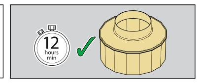
Ensure all pipework and electrical entries have been completed before vacuum testing, this is a final test for all penetrations in the sump.
