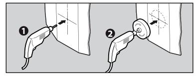
For larger holes (190mm) we recommend that the hole is marked and jigsaw is used to cut the hole. Firstly, drill a hole through the wall, so the jigsaw can be inserted and used easily and safely. (Fibreglass will blunt normal blades very quickly, we recommend diamond tipped blades or blades to cut ceramics).
