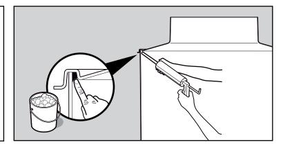
Seal around the outside joint and smooth off sealant with soapy water.
