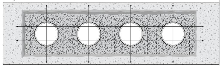
Place the corbel onto the sump (only 'dry fit' the corbel do not bond at this stage). Check the measurement from the top of the corbel to the string line, which is set 10mm above the general grade level. Check all sides of the sump and select the largest and smallest measurement to take account of falls across the forecourt.
