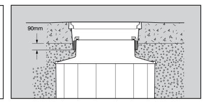
Complete backfilling to appropriate level. Frame must be supported by a minimum depth of 200mm of concrete Concrete ties must be inserted as close to the frame as possible. Minimum block of 500mm square around the frame. Joint must be tied as per diagram. Continuous pour preferred if possible.
