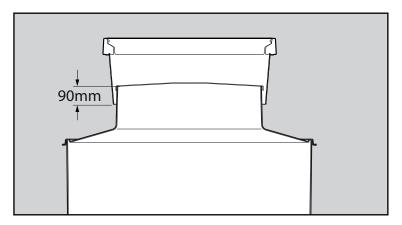
**WARNING** Do not trim sump until sump has been vacuum tested with pipework installed and completed.
