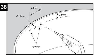
Mark out the position of the two holes to be drilled 24mm down from the top edge of the Corbel and 60mm cross centre. Drill the two Ø7mm holes into the Corbel walls.
