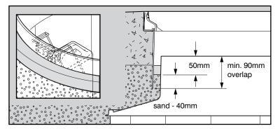
Drain and bottle should be positioned away from pipe risers and stp. The drain must be installed at the created low point to do this. Compact the sand in a way to create a low point 10-15mm lower than the surrounding sand.
